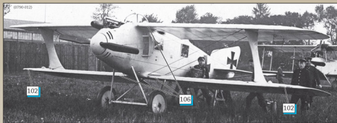
Late production Roland C.II being prepared for flight. Note the data plates on the bottom wings 102 and wing inspection stamps 106 .
