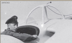
Roll over hoop detail from the Roland C.II shown on page 25.
