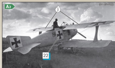
Two images reportedly showing Eduard Ritter von Schleich in his 'light blue and white' Roland C.II A2 now with the fishy anemometer fairing A11 . Looking at these photos it would appear that the light blue was very roughly applied in a 'scumble' finish over most of the aircraft but the area of the top wings inboard from the cross fields were doped white.
