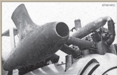
Orcarina exhaust detail from Oblt Link's elaborately checked and striped late production FFA 18 Roland C.II "Meerkatz" (not early production C.II "Meerkatz" B ). Note the oil tank filler tube visible underneath the exhaust.
