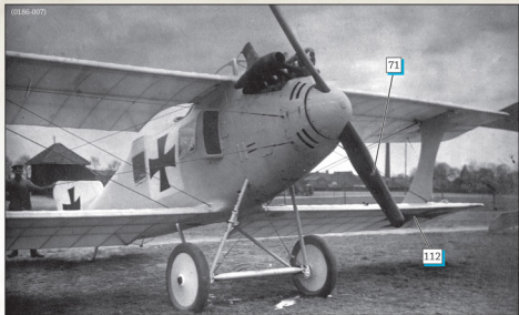
Another anonymous early production Roland C.II with translucent wing fabric, probably bleached (white) linen as opposed to CDL due to the apparent lack of a white field behind the cross on the bottom wing.
