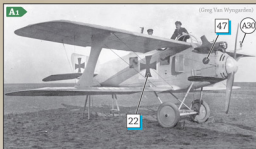
Two views of Roland C.II A1 after having a rear view mirror F1 attached to the rollover hoop shortly after arriving at FFA 2b. The anemometer has not yet received its fishy covering A11 . The original caption to the photo on the right identifies the crew as Eduard Ritter von Schleich and Vogeley, who appear to have returned from a successful photographic reconnaissance flight.
