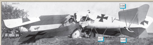
The fatal crash of von Persch's Kasta 5, Kagohl 1 Roland C.II allows us to see the drainage holes and markings on the bottom of the fuselage. The rudder cross style and low control horn position indicate an early production C.II. It would appear that the fuselage cross has been repainted mid-way between the observer and the tailplane removing the convenient aiming point between the cockpits.
